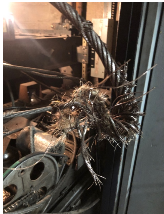
Fig. 1: When an elevator hoist rope fails
