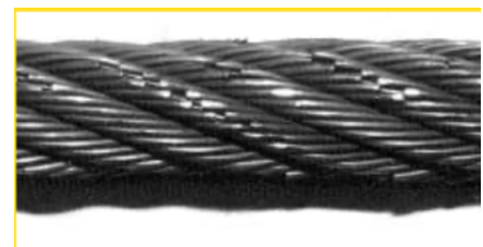
Fig. 7: Crown fatigue breaks
